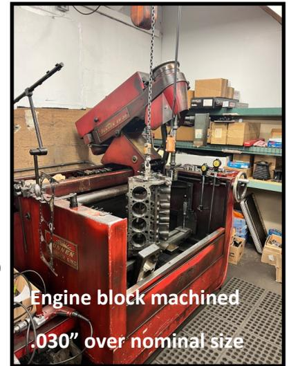
Engine block machined
